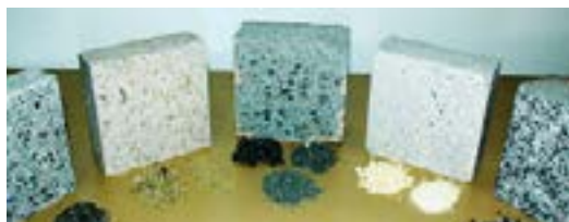
Lightweight concrete with recycled aggregates (RAEE, PU, plastics of discard from MSW, tyre rubber) for thermo-acoustic insulation
